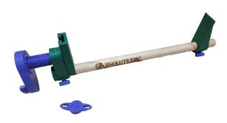
The ABSOLUTE EMC Bar Clamp is specifically designed for the EMC market, providing a low-cost, easy-to-use solution with no metallic parts. It is highly adjustable, reliable, and ideal for various EMC testing applications. The EMC Bar Clamp is made from low permittivity materials, making it suitable for holding tables together or securing the **DUT/EUT** in position during testing.
